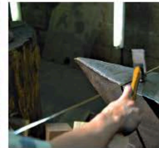
Hot forging (left) and cold hammering (right) are performed with the naked eye by experienced craftsmen. © Blaise Frères
