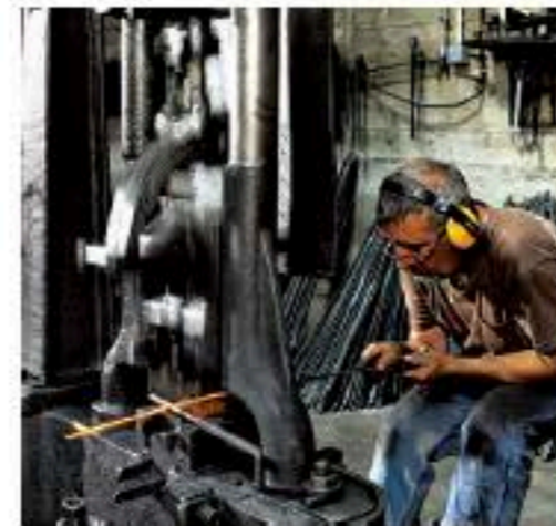
Hot forging (left) and cold hammering (right) are performed with the naked eye by experienced craftsmen. © Blaise Frères
