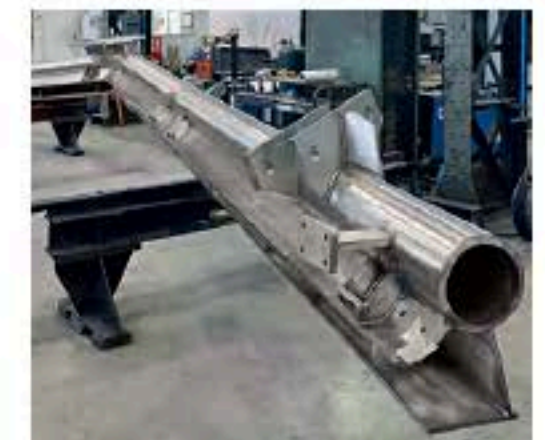
Straight or curved, duplex gutters are fitted with fixing "ears" and mounting plates. © Gérard Tordjman
